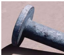
21" flanged-end open upset forging
