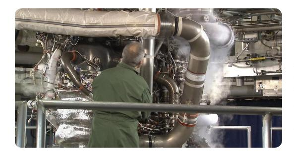
NASA engineers at Stennis Space Center near Bay St. Louis, Mississippi, took a major step Dec. 11 towards hotfire testing of RS-25 rocket engines that will help power the SLS on missions to deep space destinations. A-1 Test Stand operators at Stennis completed a chill test of developmental engine No. 0525, clearing the way for hotfire testing to begin in 2015. A chill test is a full dress rehearsal for hotfire testing. More information can be found here. (NASA/Stennis)
